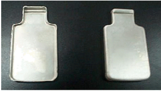
Figure 13. Micrograph of prototype sheet metal parts of the cellular phone case made by warm forming using quasicrystal strengthened Mg–Zn–Y alloys.
